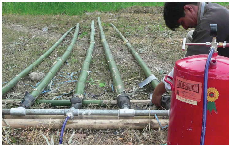
Photo 27: Bamboo boucherie treatment Photo source: INBAR, 2019 https://www.inbar.int/ .
