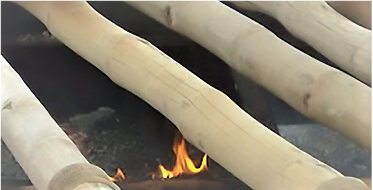
Photo 25: Drying bamboo by baking (Photo source: guaduabamboo.com ; 2019)
