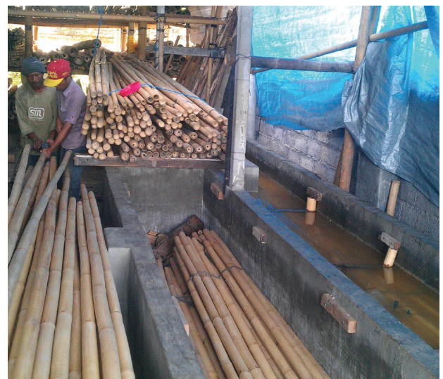
Photo 22: Soaking bamboo in water or leaching Photo source: bellobamboo.com , 2019
