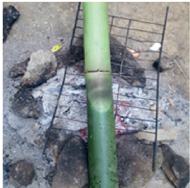
Photo 24: Drying bamboo by smoking
